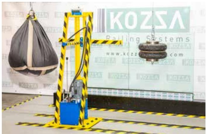
Public spaces and stadiums, where lot of people may assemble in small space, require robust balustrades. Glass thickness and heavy profiles provide safety under heavy loads. The glass balustrade must be able to withstand up to 3 KN per linear meter.
