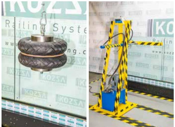
continue to exercise its function under the application of a punctual load of  $200 \text{ N} = 20 \text{ kgf}$  for 30 seconds. The impact body must not pass through the balustrade upon impact.
